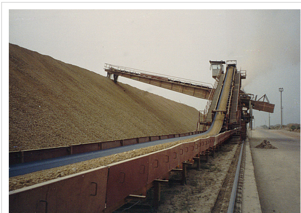
A limestone prehomogenization pile being built by a boom stacker
