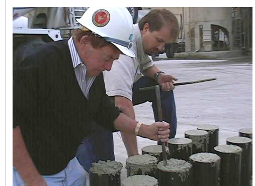
Sampling fast set concrete made from Portland cement
